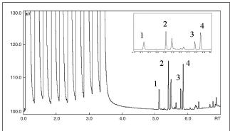
**Figure 17.** Stack injection technique on a 10-m × 0.53-mm CP-Lowox: (A) 1 injection at 50°C, followed by temperature program to 200°C and (B) 10 injections at 50°C, followed by temperature program to 200°C. Sensitivity enhancement of a factor 10. (1) Acetaldehyde, (2) propanal, (3) methanol, and (4) acetone.
