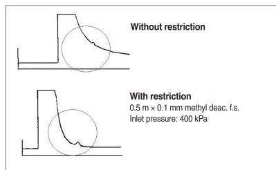
**Figure 20.** Using a restriction at the front of the 0.53-mm column allows injection at higher inlet pressure, resulting in improved peak shape.
