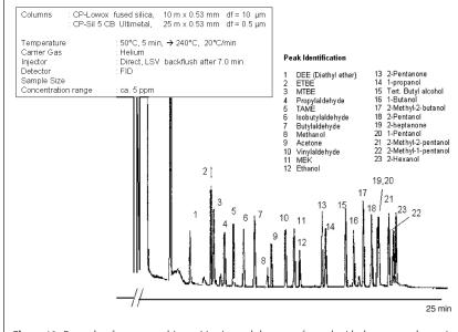
**Figure 19.** Example of oxygenated impurities in naphtha as performed with the system shown in Figure 18; besides methanol, a large range of oxygenated compounds can be determined.
