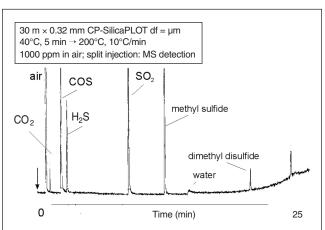
**Figure 8.** Separation of sulfur compounds on a silica PLOT column; COS and H<sub>2</sub>S elute at high temperature and are well resolved. Also, SO<sub>2</sub> shows good peak shape.
