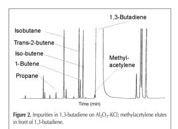
For the majority of applications, the KCl-deactivated alumina can be used. This column, which now is also recommended in several methods standardized by the American Standards Testing Materials, will separate the majority of the  $C_1$ – $C_4$  hydrocarbons and is ideal for impurity analysis (Figure 2).
