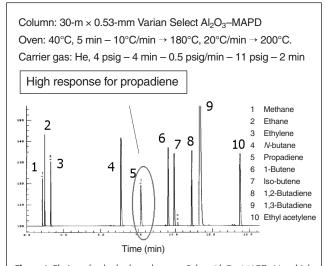
**Figure 4.** Elution of polar hydrocarbons on Select-Al<sub>2</sub>O<sub>3</sub>–MAPD. Note high response for acetylene and propadiene (courtesy of J. Luong, Dow *Chemical, Canada*).
