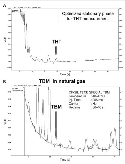
**Figure 14.** Fast analysis of odorants in natural gas using the CP4900 micro GC: analysis of THT (A) and analysis of TBM (B).
