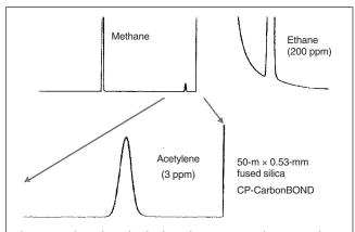
**Figure 5.** Analysis of ppm levels of acetylene on a CP-CarboBOND column. Acetylene elutes before ethylene. Symmetrical peak allows sub-ppm level determination (courtesy of J. Luong, Dow Chemical, Canada).
