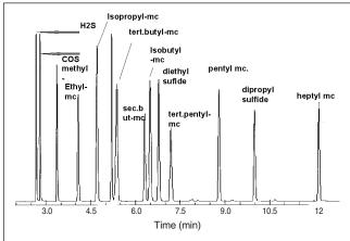
**Figure 7.** Separation of most common sulfur compounds on thick-film PDMS (CP-Sil 5 CB) using SCD detection (courtesy of J. Luong, Dow Chemical, Canada).
