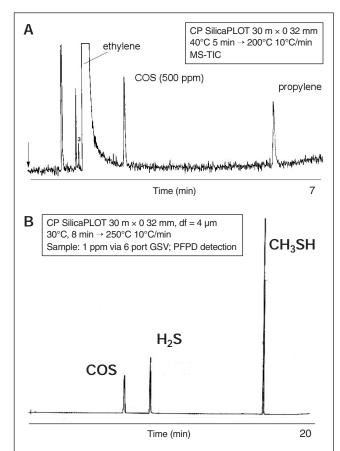
**Figure 9.** (A) Separation of COS and propylene on a silica PLOT column; COS is well resolved from propylene allowing ppb-level detection with selective detectors. (B) Determination of trace COS in propylene matrix; no quenching is possible, as COS is well separated from propylene.
