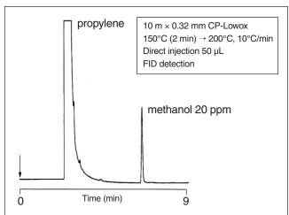
Figure 15. Analysis of methanol on propylene with 10-m  $\times$  0.53-mm CP-Lowox.
