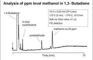
Figure 16. Analysis of methanol in 1,3-but adiene using 10-m  $\times$  0.53-mm CP-Lowox.
