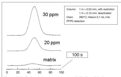
**Figure 13.** Total sulfur determination using a  $1 \text{-m} \times 0.53 \text{-mm}$  CP-Sil 5 CB coupled with a  $1 \text{-m} \times 0.1 \text{-mm}$  deactivated fused silica (courtesy of Aviv Amirav, University Tel Aviv).
